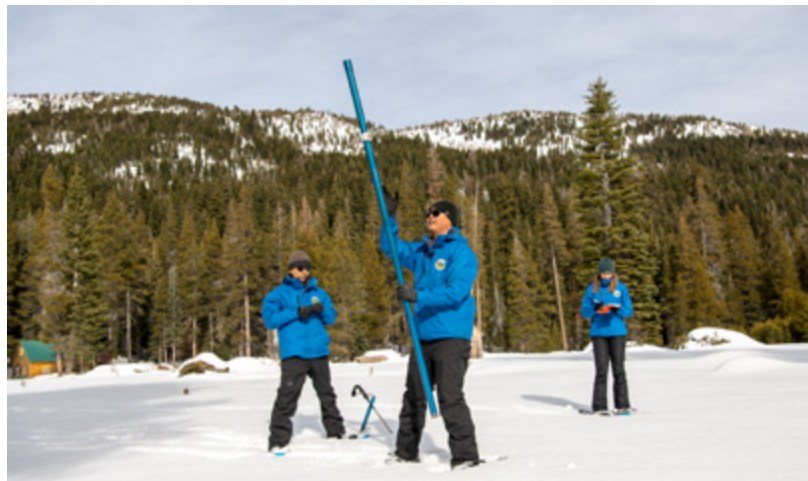
The first manual survey of the year shows snow 33.5 inches deep at Phillips Station in the Sierra. The snow water equivalent of 11 inches is 97% of average for the location.
