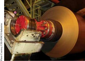
The manufacture of cold rolled annealed steel on the Kawasaki Multipurpose Continuous Annealing Line at USS-POSCO Industries.
