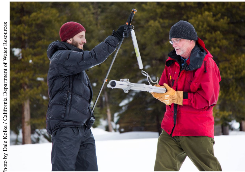
Mikel Shybut (left), science policy fellow with the California Council on Science and Technology, helps Frank Gehrke, chief of the California Cooperative Snow Surveys Program, with the second snow survey of the 2017 season on February 2 at Phillips Station in the Sierra Nevada. The survey site is about 90 miles east of Sacramento off Highway 50 in El Dorado County.
